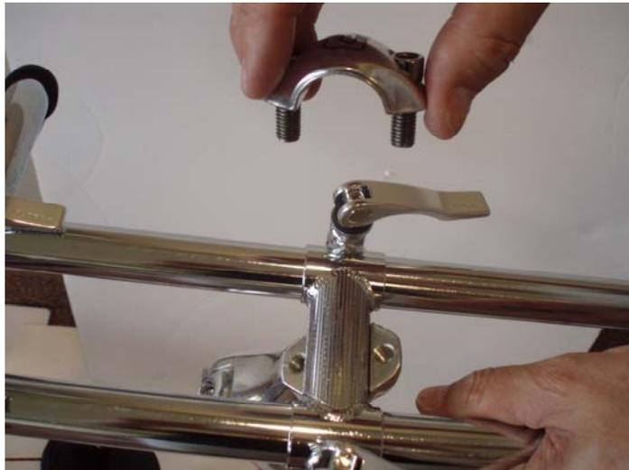
d) Tighten 2 hex head screws at top of stem to tighten Handlebar clamp.
