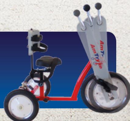
Hinged Front End with 3 Positions for adjustable hand crank/ foot crank to seat alignment
